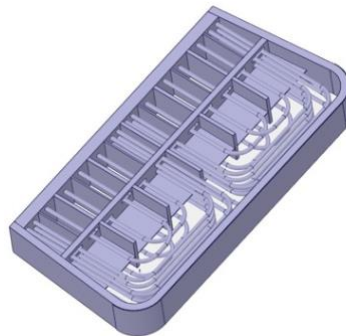
Fig. 1: WCLL inboard BU: perspective view of the Inboard breeding unit showing the inner cooling pipes layout.
