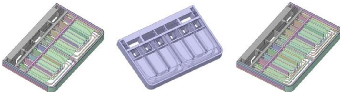
Fig. 2: WCLL inboard BUs: perspective view of the Inboard breeding unit showing the inner cooling pipes layout (from left to right: 'alt. 22', 'v06b' and 'alt.24' concepts).
