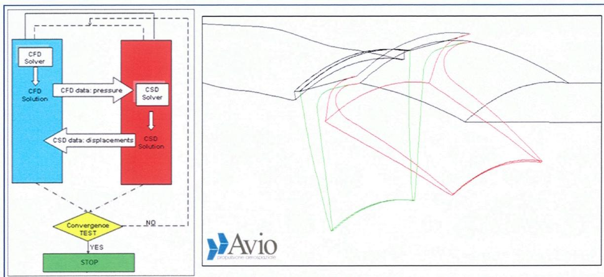
*Figure 3 : FSI Flow chart and PTF deformations.*
